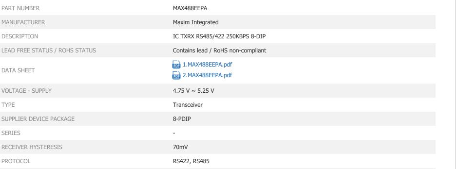
**PACKAGING** Tube PACKAGE / CASE 8-DIP (0.300", 7.62mm)
