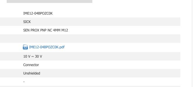
RESPONSE FREQUENCY 2kHz Cylinder, Threaded - M12 PACKAGE / CASE **OUTPUT TYPE** PNP-NC, 3-Wire
