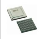
**89HPES6T6G2ZCALGI** Manufacturers: IDT (Integrated Device Technology) Description: IC PCIE SW 6LANE 6PORT 324FCBGA In stock: Out stock
