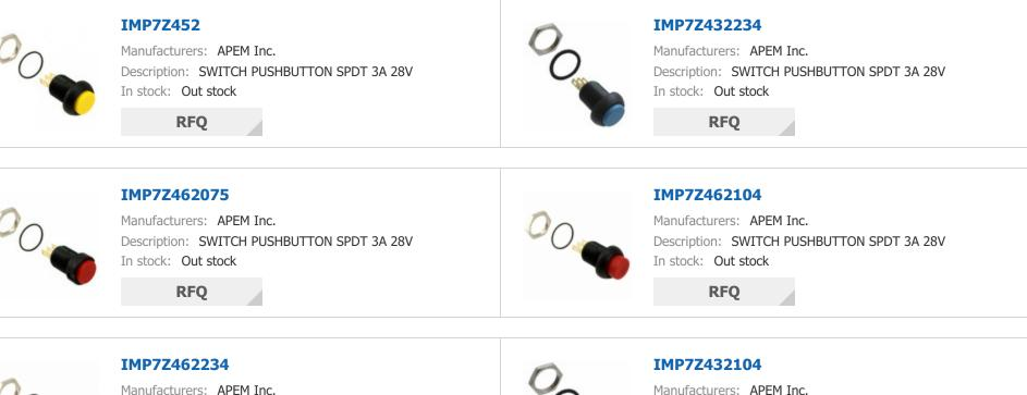
Description: SWITCH PUSHBUTTON SPDT 3A 28V In stock: Out stock
