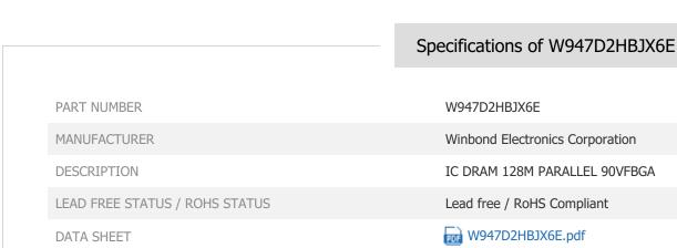
WRITE CYCLE TIME - WORD, PAGE **VOLTAGE - SUPPLY** 1.7 V ~ 1.95 V **TECHNOLOGY** SDRAM - Mobile LPDDR SUPPLIER DEVICE PACKAGE 90-VFBGA (8x13) **SERIES PACKAGING** Tray 90-TFBGA PACKAGE / CASE -25°C ~ 85°C (TC) OPERATING TEMPERATURE MOUNTING TYPE Surface Mount MOISTURE SENSITIVITY LEVEL (MSL) 3 (168 Hours) MEMORY TYPE Volatile 128Mb (4M x 32) MEMORY SIZE **MEMORY INTERFACE** Parallel
