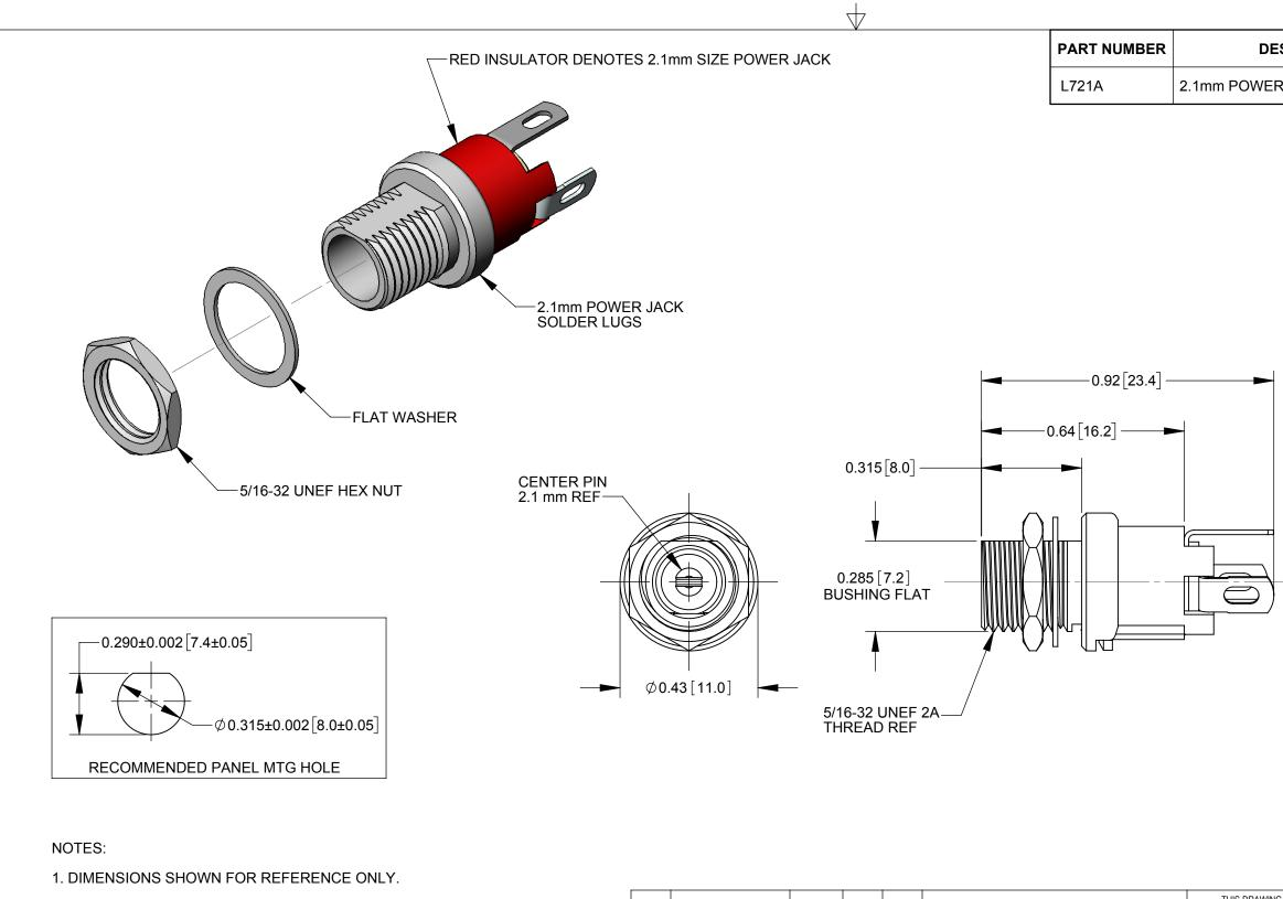
2. HEX NUT AND FLAT WASHER SUPPLIED UNASSEMBLED.
