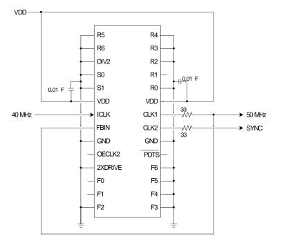
Note: The series termination resistor is located before the feedback trace. This will give the following waveforms:
