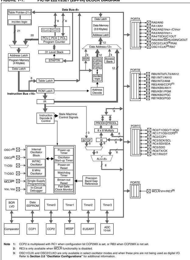
FIGURE 1-1: PIC18F2221/2321 (28-PIN) BLOCK DIAGRAM
