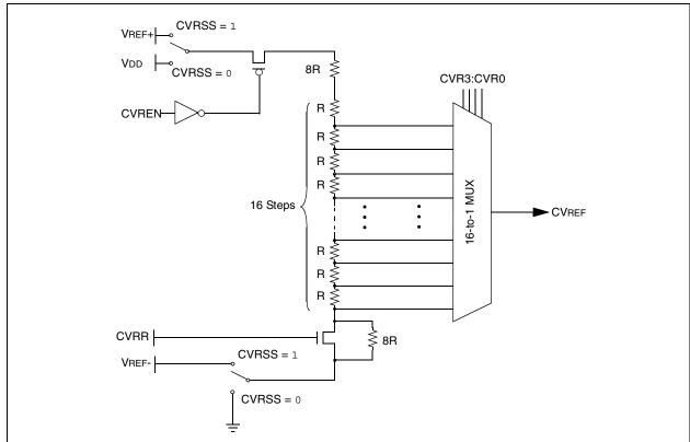
FIGURE 21-1: COMPARATOR VOLTAGE REFERENCE BLOCK DIAGRAM
