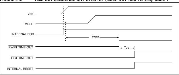
FIGURE 4-5: TIME-OUT SEQUENCE ON POWER-UP (MCLR NOT TIED TO VDD): CASE 2
