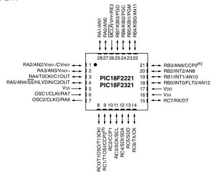
Note 1: RB3 is the alternate pin for CCP2 multiplexing.
