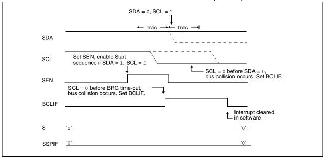
FIGURE 17-30: BRG RESET DUE TO SDA ARBITRATION DURING START CONDITION
