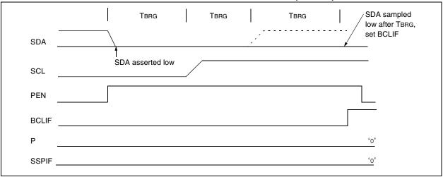
FIGURE 17-34: BUS COLLISION DURING A STOP CONDITION (CASE 2)
