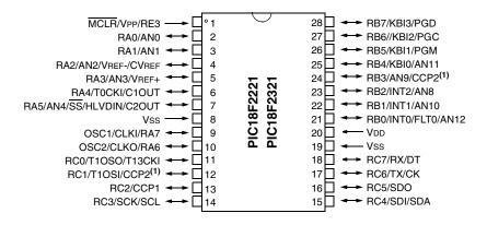
Note 1: RB3 is the alternate pin for CCP2 multiplexing.
