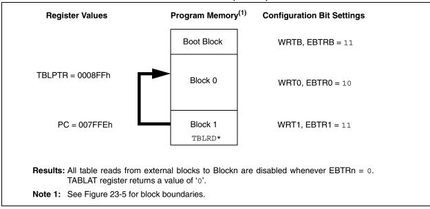
FIGURE 23-8: EXTERNAL BLOCK TABLE READ (EBTRn) ALLOWED
