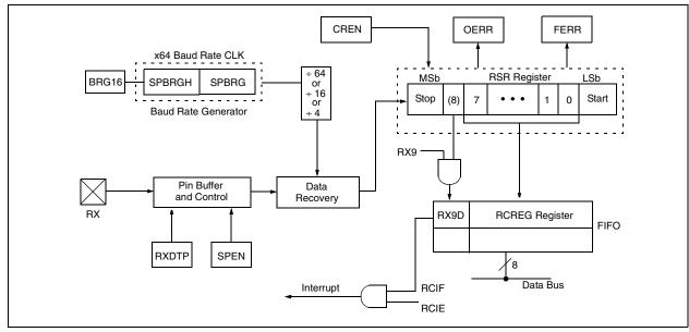
FIGURE 18-7: ASYNCHRONOUS RECEPTION, TXCKP = 0 (TX NOT INVERTED)
