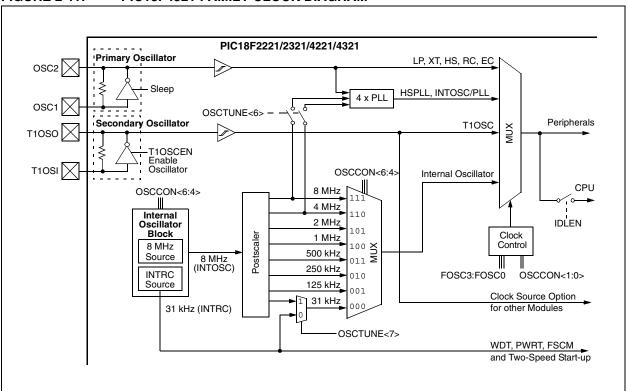
FIGURE 2-11: PIC18F4321 FAMILY CLOCK DIAGRAM
