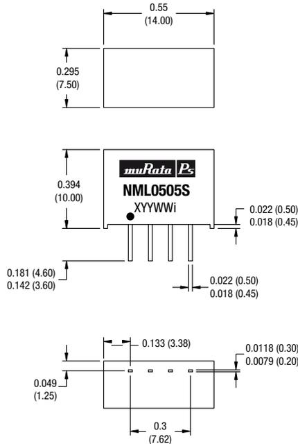
All dimensions in inches  $\pm 0.01$  (mm  $\pm 0.25$ mm). All pins on a 0.1 (2.54) pitch and within  $\pm 0.01$  (0.25) of true position.
