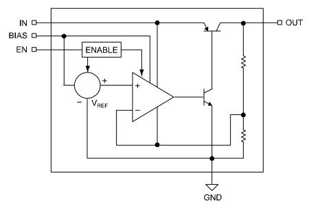
**Block Diagram – Fixed Output Voltage**
