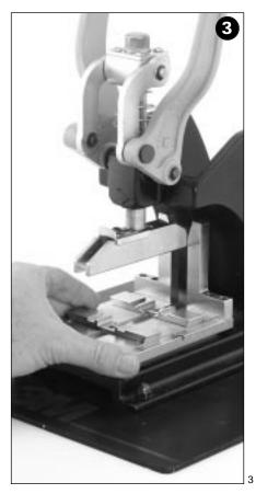
Install the 10981-5 platen and the locator plate on the press.
