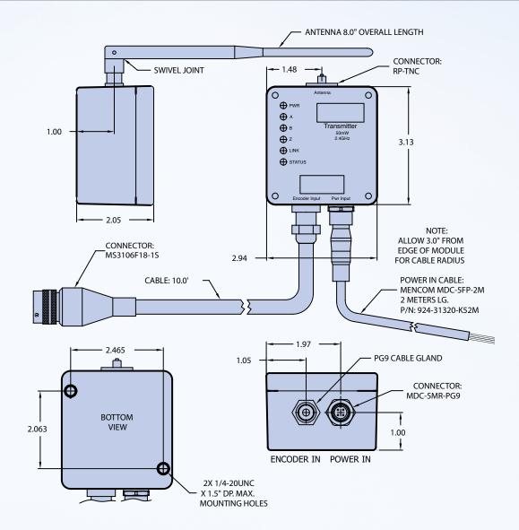
The SwiftComm Transmitter Module has two connector plugs: a 5-pin connector for power input, B.I.T output and chassis ground; and a 3-meter cable with a 10-pin MS connector attached to the end.
