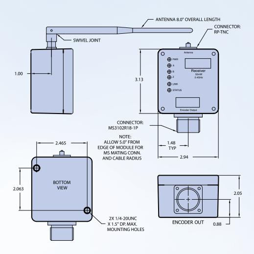
The SwiftComm Receiver Module has an MS connector that provides the same output signals as a standard BEI encoder.
