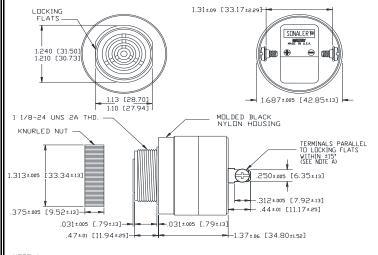
NOTE A: TERMINALS-.032 BRASS TIN PLATED, TAPPED FOR #6-32 SCREW. TWD #6-32 NICKEL PLATED BRASS SCREWS INCLUDED. WILL ACCEPT 1/4\* QUICK CONNECT.
