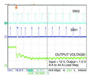
Figure 9. Load Transient with 2 Phases
