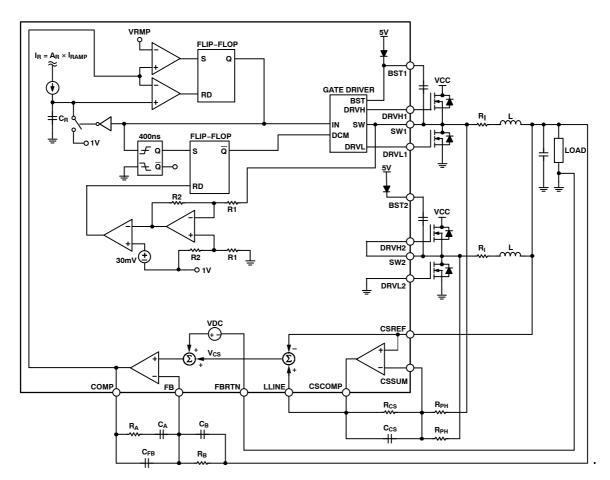
Figure 26. Single-Phase RPM Mode Operation
