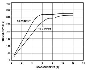
Figure 39. Single-Phase CCM/DCM Frequency vs.
