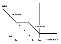
Figure 44. Poles and Zeros of Voltage Error Amplifier
