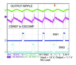
Figure 10. Switching Waveforms in 2 Phase
