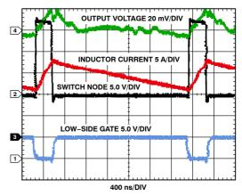
Figure 32. Single-Phase Waveforms in CCM
