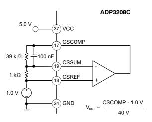
Figure 2. Closed-Loop Output Voltage Accuracy
