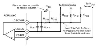
Figure 42. Temperature-Compensation Circuit **Values**
