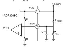
Figure 45. Single-Point Thermal Monitoring
