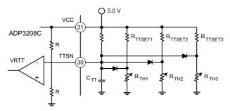
Figure 46. Multiple-Point Thermal Monitoring
