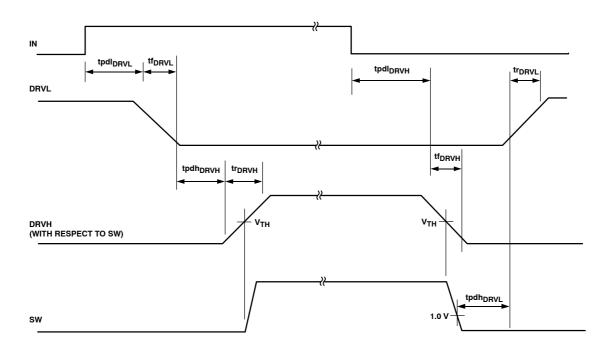
Figure 6. Timing Diagram (Note 3)
