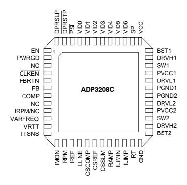
Figure 5. Pin Configuration (Top View)
