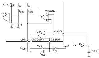
Figure 30. Current Limit Circuit
