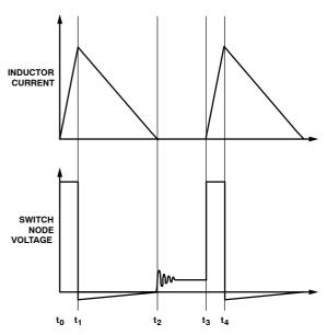
Figure 37. Inductor Current and Switch Node in DCM
