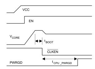
Figure 29. Powerup Sequence of ADP3208C
