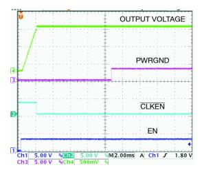
Figure 18. Startup Waveforms
