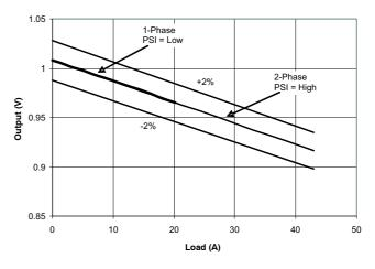
Figure 16. Load Line Accuracy
