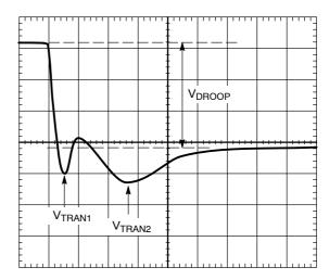
Figure 48. Transient Setting Waveform, Load Step
