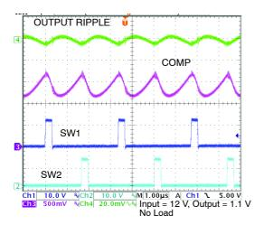
Figure 11. Switching Waveforms in 2-Phase
