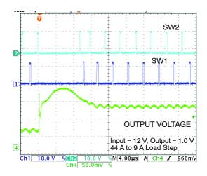
Figure 8. Load Transient with 2-Phases
