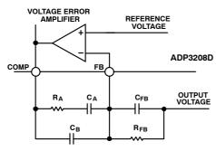
Figure 43. Voltage Error Amplifier
