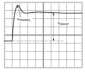
Figure 49. Transient Setting Waveform, Load Release
