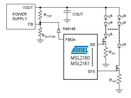
Figure 5. FBOn Connects to the Power Supply Voltage Divider Through a Diode.
