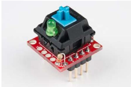
In addition to breaking out the switch contacts to breadboard-compatible headers, the breakout also provides access to an optional switch-mounted LED. Plus, the pin break-outs are designed with keyboard matrix-ing in mind, so you can interconnect as many boards as you'd like into a row-column configuration, keeping the I/O-pin requirements as low as possible.
