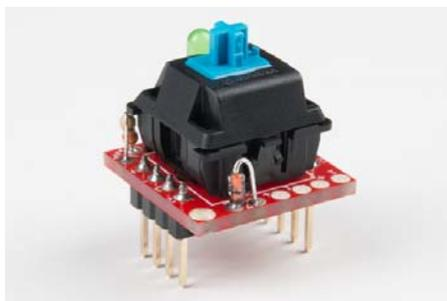
You'll also need to **cut the "D" jumper** on the back side of the board – otherwise the diode will be shorted over. (This may be easier if you do it before soldering anything.)
