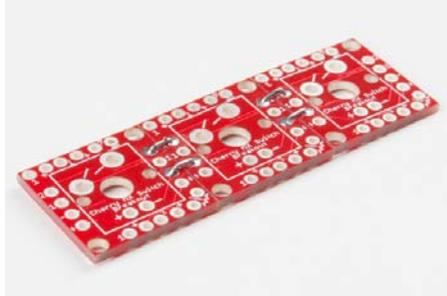
There's not an easy method to soldering boards together. You'll probably need wire strippers to split and cut solid-core wire into tiny (~3/8") pieces. A third hand can be a big-time help keeping boards stationary while you solder the little wires in place.
