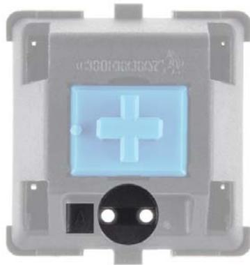
*The LED's recessed home in the switch. Note the “A” indicator for the LED's “anode.”*
