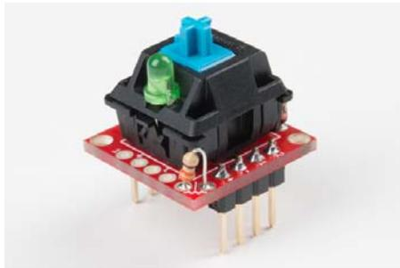
You'll also need to **cut the "R" jumper** on the back side of the board, which might be easier to do before you solder anything. A hobby knife and a steady hand should do the trick.
