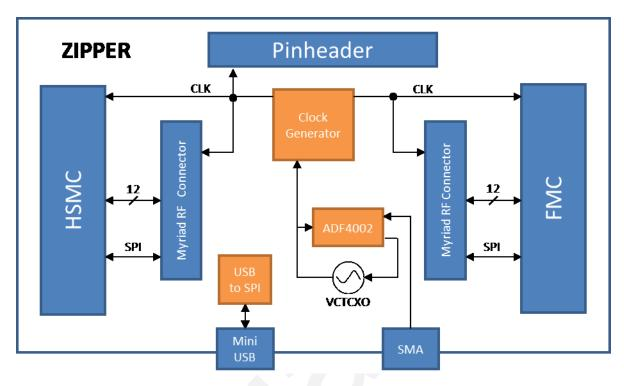
Figure 2. Zipper board block diagram.
