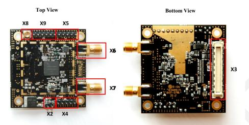
Figure 29. Myriad-RF board connection descriptions.
