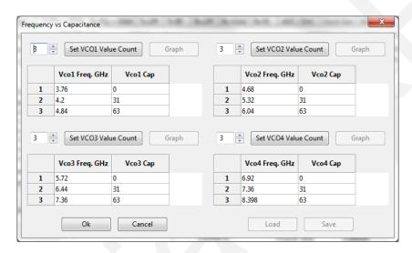
Figure 18. Frequency vs capacitance calibration table data
