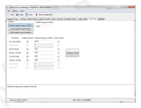
Figure 27. Control window for on board clock generator.
