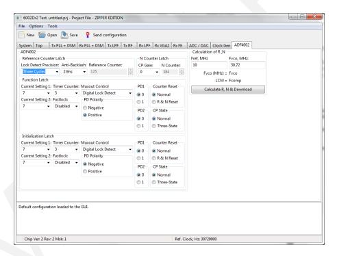
Figure 28. Control window for on board ADF4002.
