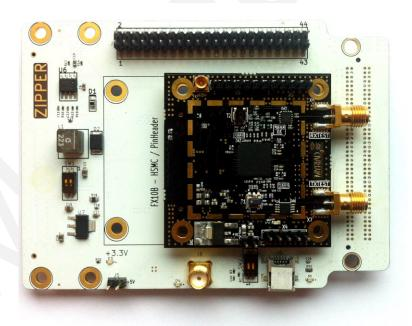
Figure 1. Zipper and Myriad-RF board development system
