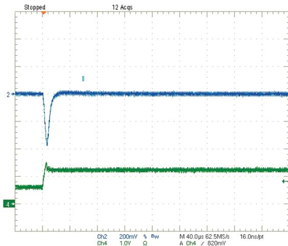
Step Load Transient Response (Vin=12V, Vout=1.0V, Load=0, Iout=6A to 3A)
