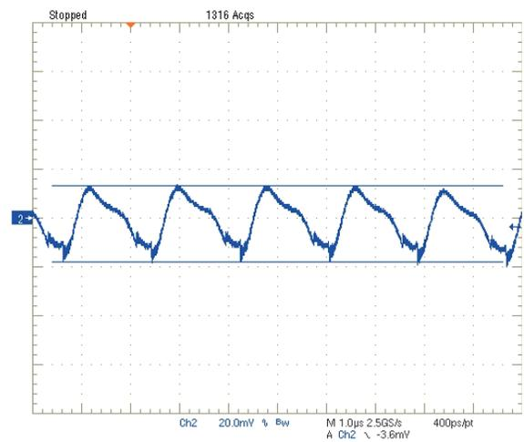
Step Load Transient Response (Vin=12V, Vout=1.8V, Load=0, Iout=3A to 6A)
