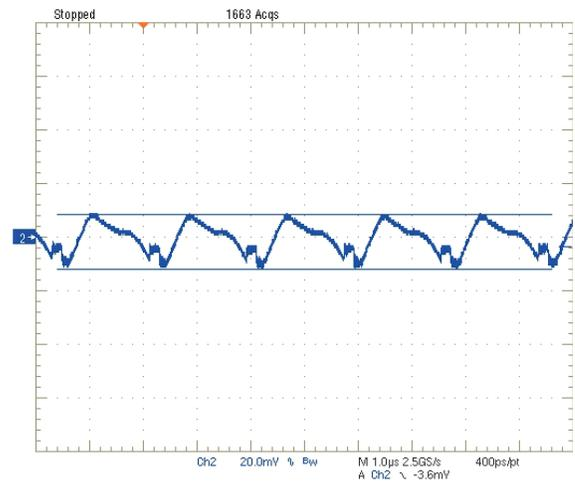
Step Load Transient Response (Vin=12V, Vout=1.0V, Load=0, Iout=3A to 6A)
