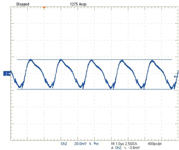
Step Load Transient Response (Vin=12V, Vout=2.5V, Load=0, Iout=3A to 6A)
