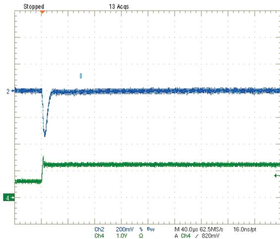
Step Load Transient Response (Vin=12V, Vout=1.8V, Load=0, Iout=6A to 3A)
