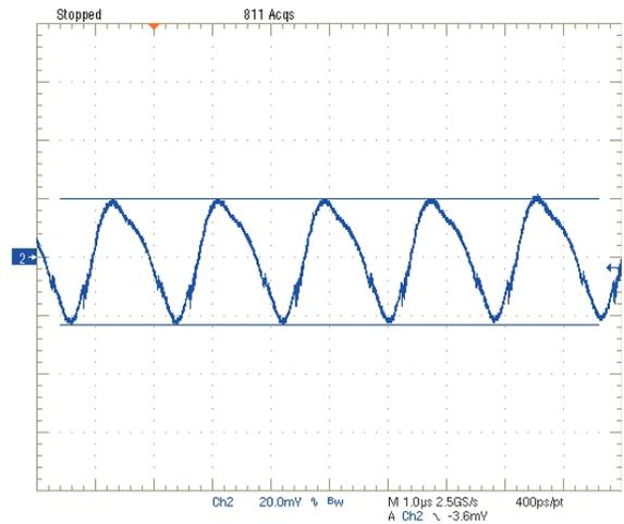
Step Load Transient Response (Vin=12V, Vout=3.3V, Load=0, Iout=3A to 6A)
