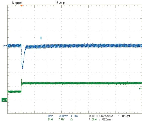
Step Load Transient Response (Vin=12V, Vout=3.3V, Load=0, Iout=6A to 3A)
