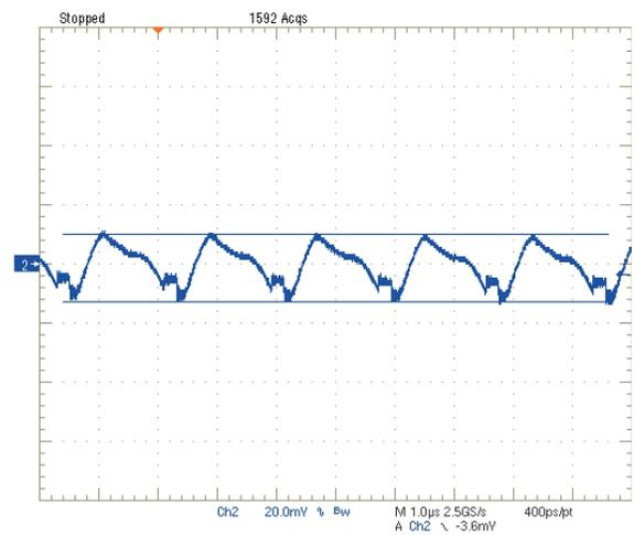
Step Load Transient Response (Vin=12V, Vout=1.2V, Load=0, Iout=3A to 6A)
