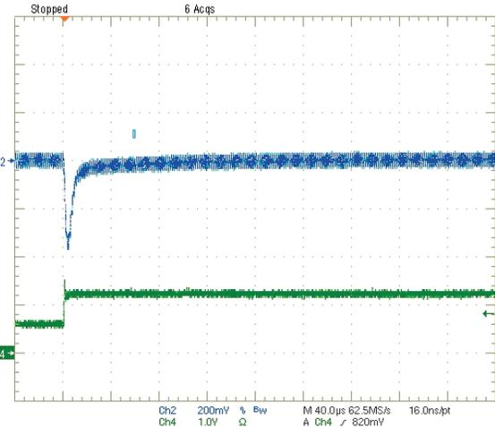
Step Load Transient Response (Vin=12V, Vout=5.0V, Load=0, Iout=6A to 3A)
