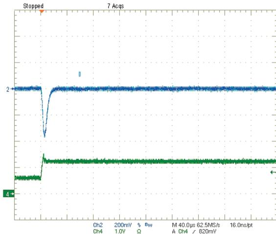
Step Load Transient Response (Vin=12V, Vout=1.2V, Load=0, Iout=6A to 3A)
