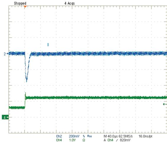
Step Load Transient Response (Vin=12V, Vout=2.5V, Load=0, Iout=6A to 3A)
