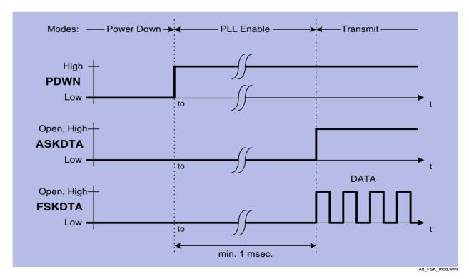
Figure 3-9 Alternative FSK Modulation
