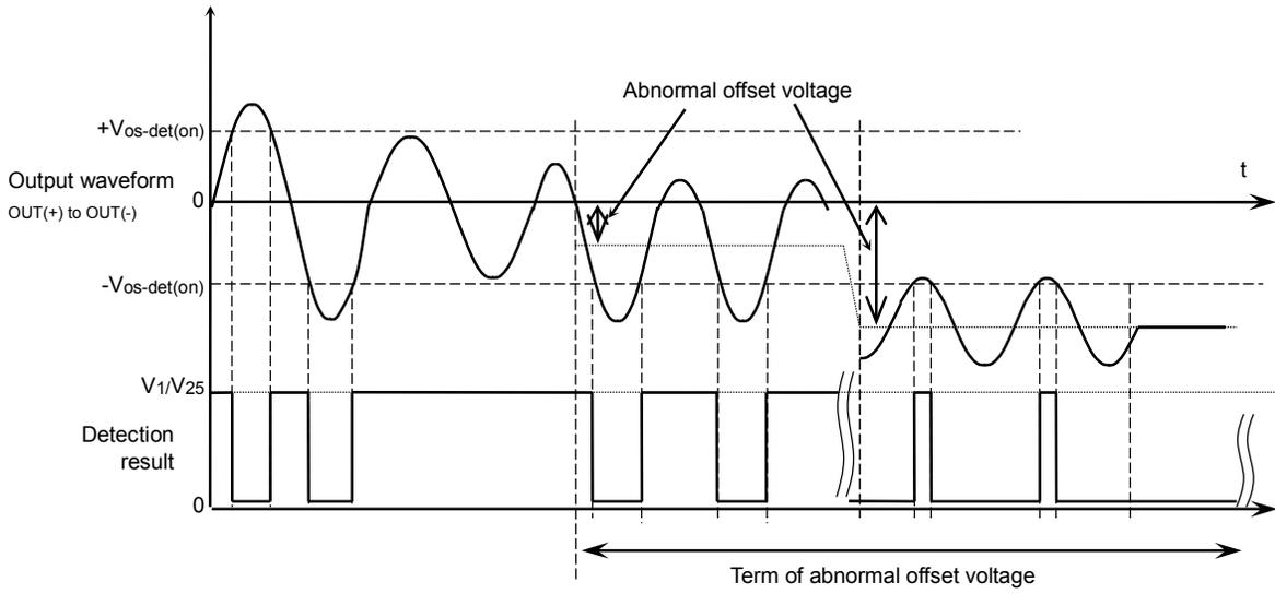
Figure 8 The detected result and audio output waveform
