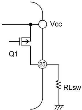
Figure 6 High-side Switch
