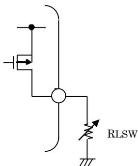
High side switch test circuit 1
