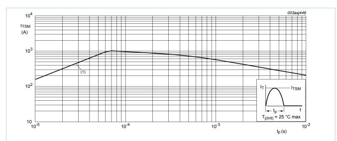
Fig. 5. Non-repetitive peak on-state current as a function of pulse width for sinusoidal currents; maximum values  $t_p \leq 10 \; ms; \, (1) \; dI_T \, / \; dt \; limit$
