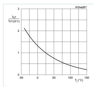
Fig. 7. Normalized gate trigger current as a function of Fig. 8. junction temperature
