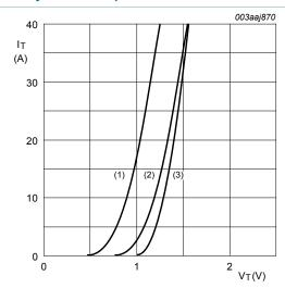
$V_o$  = 1.0336 V;  $R_s$  = 0.0141  $\Omega$ (1) T<sub>i</sub> = 150 °C; typical values
