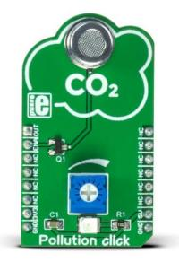
**Pollution click** has high sensitivity to organic gases such as methanal (also known as formaldehyde), benzene, alcohol, toluene, etc. The click carries the WSP2110 VOC gas sensor with the detection range of  $1 \sim 50$  ppm (parts per million).
