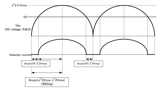
Given that the ratio of inductor current to AC input is DutyAC.
