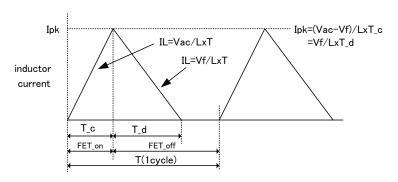
Given that the period when current flows into coil is
