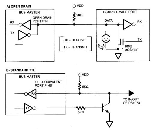
Programming mode is entered by simply powering up the DS1073 with a pullup of approximately  $5k\Omega$ . This will pull the I/O pin above V<sub>IH</sub> on power-up and initiate the programming mode, causing the DS1073 to internally release the I/O pin (after t<sub>POR</sub>), and allow the pullup resistor to pull the pin to the supply rail and await the Master Tx Reset pulse (see diagram).
