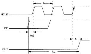
$t_M$  = PERIOD OF MCLK  $t_d$  = PROP DELAY FROM MCLK  $\uparrow$  TO OUT  $\uparrow$ MAX VALUE OF  $t_{en} = t_{SUEM} + 2 t_M + t_d$ MIN VALUE OF ten =  $t_{SUEM} + t_M + t_d$
