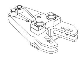
Battery Tool (Pin Die) 1213890-1, -2 (Customer Manual 409-10065)
