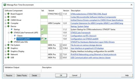
Click **Resolve** to enable other required software components and then **OK**. A new window will ask you to start **STM32CubeMX**.
