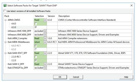
When the project is completed, disable the option **Use latest version of all installed Software Packs** and specify the software packs with the settings under **Selection**:
