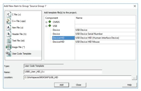
To connect the PC USB application to the microcontroller device, modify the function *USBD\_HID0\_SetReport()*, which handles data coming from the USB Host. For this example, the data is created with the utility **HIDClient.exe**.
