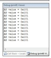
As ITM is not available in Cortex-M0/M0+ devices, you can use the event recorder to display printf debug messages. Use the **EVR** variant of the STDOUT I/O channel for this purpose (works with all Cortex-M based devices).
