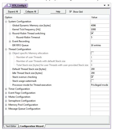
You can set parameters for the thread stack, configure the Tick Timer, set Round-Robin time slice, and define user timer behaviour for threads.
