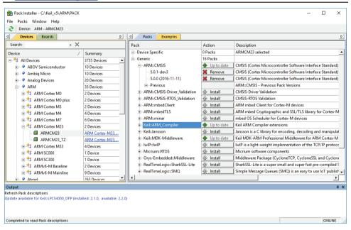
The status bar, located at the bottom of the Pack Installer, shows information about the Internet connection and the installation progress.
