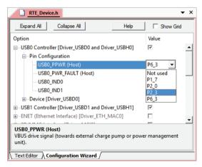
Using the **Configuration Wizard** view, you can configure the driver interfaces in a graphical mode without the need to edit manually the #defines in this header file.
