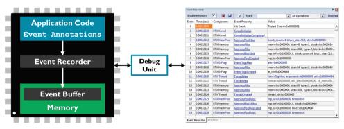
During program execution, the  $\mu$ Vision debugger reads the content of the event buffer using a debug adapter that is connected via JTAG or SWD to the CoreSight Debug Access Port (DAP). The event recorder requires no trace hardware and can therefore be used on any Cortex-M processor based device.
