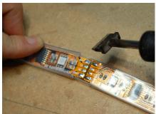
Cut the remaining rubber underneath with scissors:
