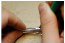
Pull off the thin rubber piece between the cuts:
