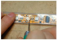
Then slice the rubber coating between the two cuts you made:
