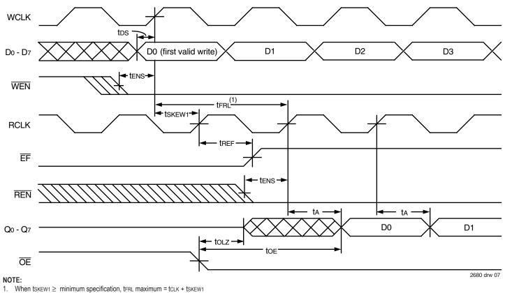
tskew1 < minimum specification, tFRL maximum = 2tCLK + tskew1 or tCLK + tskew1
