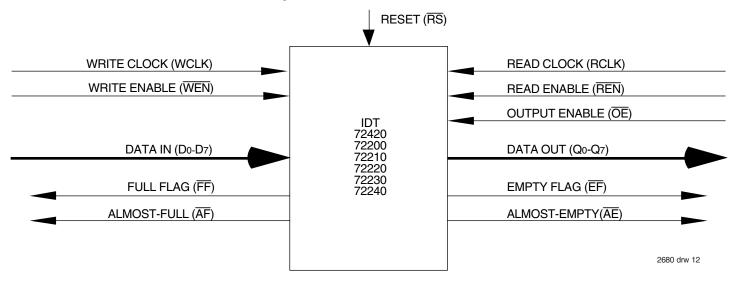
Figure 10. Block Diagram of Single 64 x 8, 256 x 8, 512 x 8, 1,024 x 8, 2,048 x 8, 4,096 x 8 Synchronous FIFO
