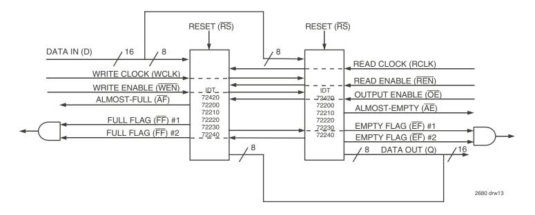
Figure 11. Block Diagram of 64 x 16, 256 x 16, 512 x 16, 1,024 x 16, 2,048 x 16, 4,096 x 16 Synchronous FIFO Used in a Width Expansion Configuration
