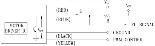
CAUTION: THE FG SIGNAL LEAD WIRE MUST BE KEPT AWAY FROM "+" LEAD WIRE & "-" LEAD WIRE.
