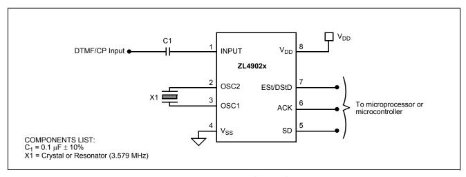
Figure 3 - Application Circuit for ZL4902x
