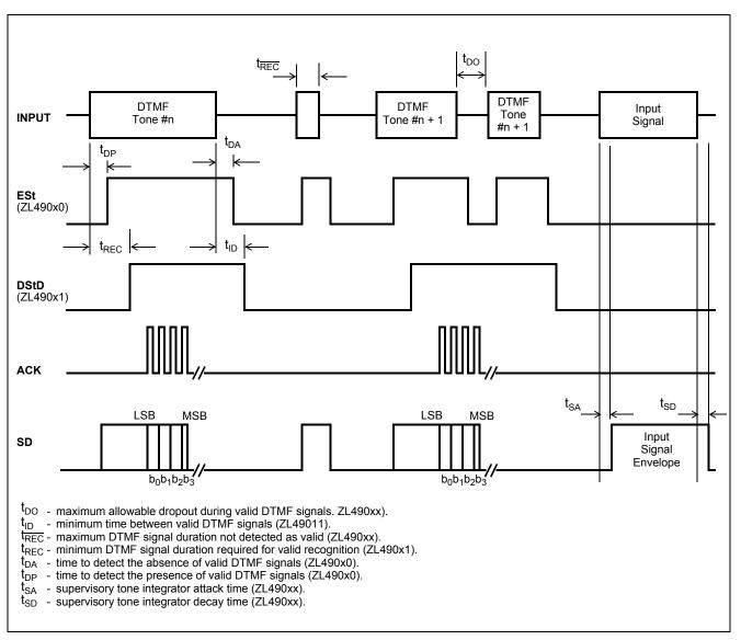
Figure 4 - Timing Diagram
