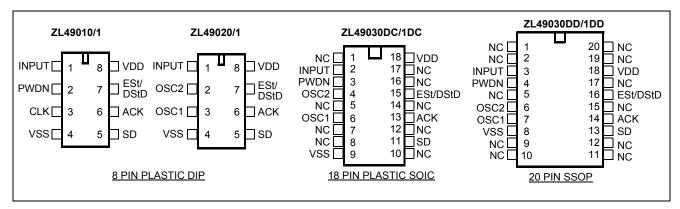
Figure 2 - Pin Connections
