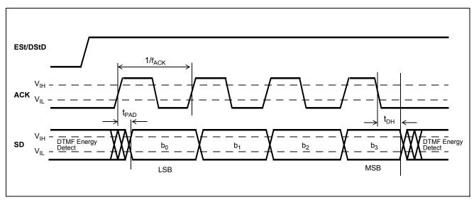
Figure 5 - ACK to SD Timing
