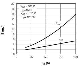
Fig. 3 - IGBT Switching Loss vs. I<sub>C</sub>
