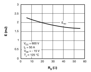
Fig. 9 - Diode Switching Loss vs. R<sub>G</sub>
