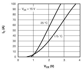
Fig. 1 - IGBT Typical Output Characteristics
