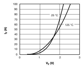
Fig. 7 - Diode Forward Characteristics
