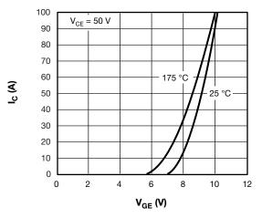
Fig. 2 - IGBT Transfer Characteristics
