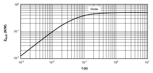
Fig. 10 - Diode Transient Thermal Impedance
