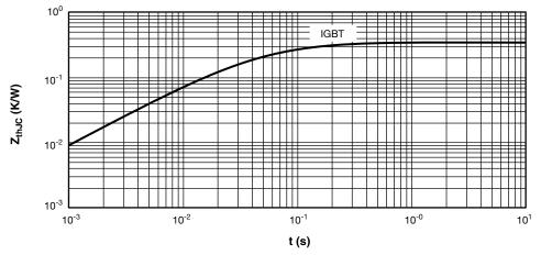
Fig. 6 - IGBT Transient Thermal Impedance
