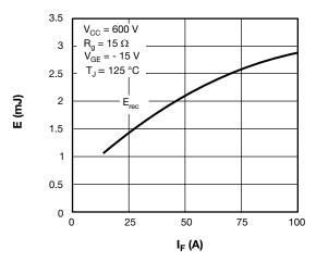
Fig. 8 - Diode Switching Loss vs. I<sub>F</sub>
