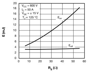
Fig. 4 - IGBT Switching Loss vs. R<sub>G</sub>
