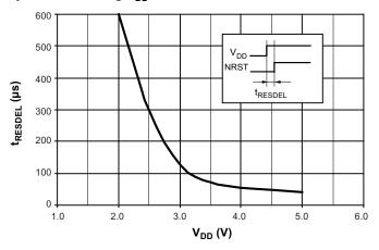
Figure 9-2. Typical Reset Delay After Switching  $\mathbf{V}_{\mathrm{DD}}$  On
