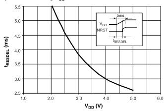
Figure 9-3.  $V_{DD}$  Rise Time to Ensure Power-on Reset
