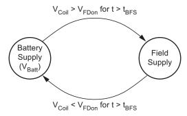
Note: The rectified supply voltage from the coil is limited to  $V_{DDC}$  (2.9V). During field supply, the battery is switched off and  $V_{DD}$  changes to  $V_{DDC}$ .
