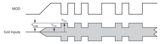
Figure 4-2. GAP and Modulation Timing
