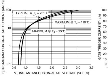
Figure 3. Typical On–State Characteristics
