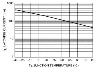
Figure 7. Typical Latching Current versus Junction Temperature
