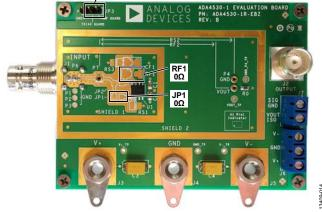
Figure 7. Buffer with Triax Guard Driven by Amp Guard
