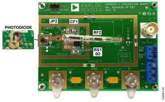
Figure 17. Transimpedance with Direct Sensor Connection
