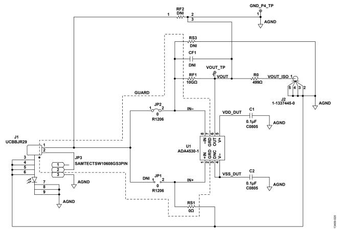
Figure 24. ADA4530-1R-EBZ-TIA Schematic
