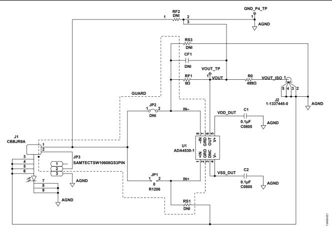
Figure 25. ADA4530-1R-EBZ-BUF Schematic
