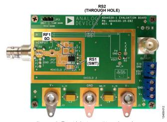
Figure 9. Buffer with Resistor at IN+ to Ground
