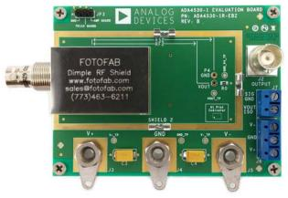
Figure 21. Evaluation Board Top View with SHIELD1
