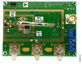
Figure 15. Transimpedance with Through Hole Feedback Resistor
