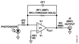
Figure 18. Transimpedance with Direct Sensor Connection Schematic
