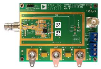
Figure 5. Buffer with Triax Guard Externally Driven
