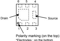
\*Electrodes: on the bottom
