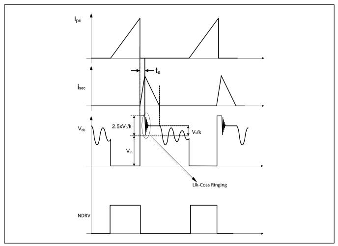
Figure 5. Waveforms with RCD Clamp.
