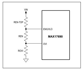
Figure 1. Programming EN/UVLO and OVI
