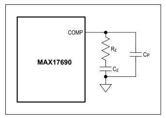
Figure 3. Loop Compensation Arrangement
