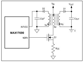
Figure 2. INTVCC Pin Configuration.
