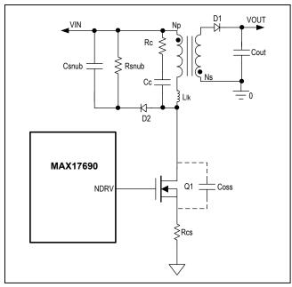
Figure 4. RC and RCD Clamp Circuitry
