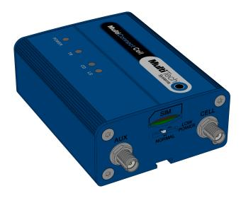
**Note:** The power-saving switch—which appears with the NORMAL and LOW POWER labels—is included only on models that have a serial connector.
