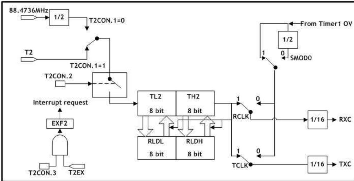
Figure 5.19 Timer2 for Baud Rate Generator Mode
