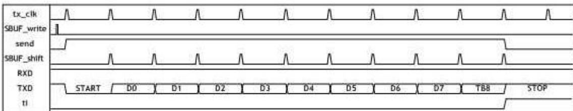
Figure 6.9 Timing Diagram for UART Transmission Mode2
