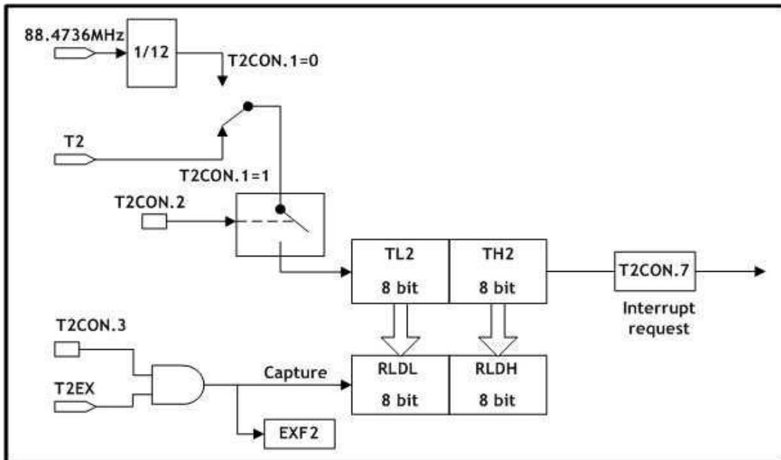
Figure 5.18 Timer/Counter2, 16-Bit Timer/Counter with Capture Mode
