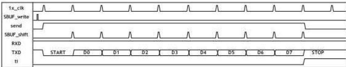
Figure 6.8 Timing Diagram for UART Transmission Mode1
