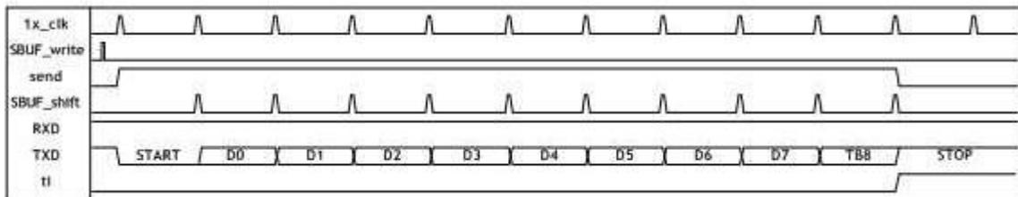
Figure 6.10 Timing Diagram for UART Transmission Mode3
