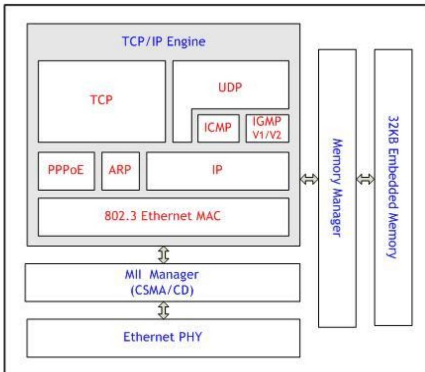
Figure 1.6 TCPIPCore Block Diagram
