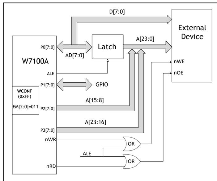
Figure 2.7 Standard 8051 External Pin Access Mode (EM[2:0] = “011”)
