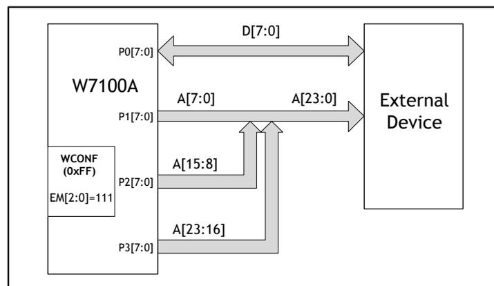
Figure 2.9 Direct 8051 External Pin Access Mode (EM[2:0] = “111”)
