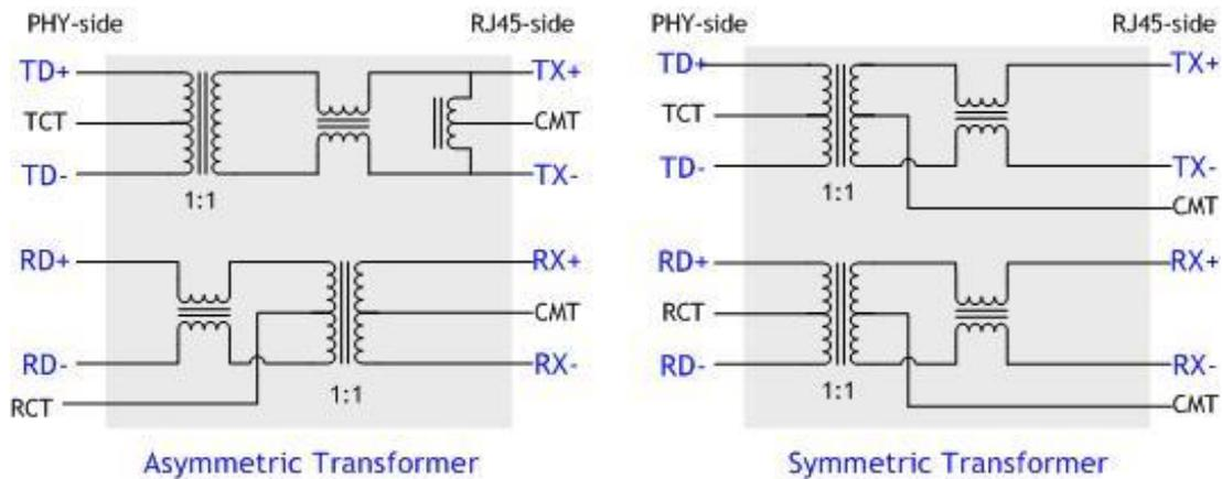
In the case of using the internal PHY mode, be sure to use symmetric transformer in order to support Auto MDI/MDIX (Crossover).
