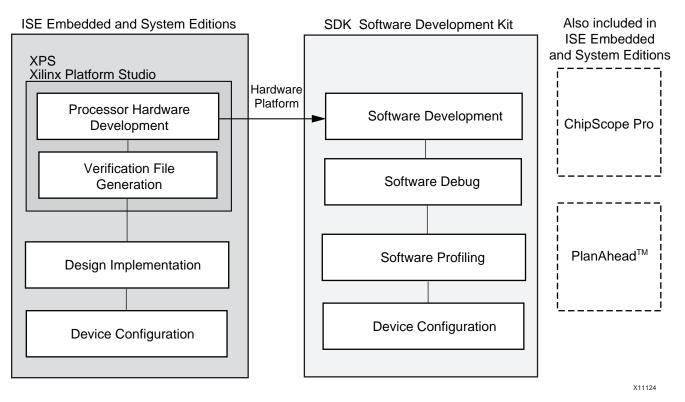
Figure 1-1: Basic Embedded Design Process Flow
