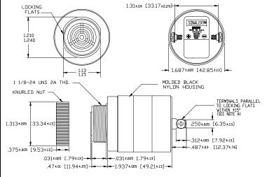
NOTE A: TERMINALS-.032 BRASS TIN PLATED, TAPPED FOR #6-32 SCREW. TWO #6-32 NICKEL PLATED BRASS SCREWS INCLUBED. WILL ACCEPT 1/4' QUICK CONNECT. NOTE B: MOUNTING- REMOVE BLACK PLASTIC NUT AND INSERT THREADED FRONT THROUGH 125' HOLE PUNCHED IN PANEL, IF DERENTATION IS NEEDED, NOTE LOCKING FLATS ON DRAVING. SCREW NUT BACK ON. DO NOT OVERTIGHTEN.
