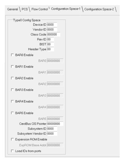
Figure 3.4. PCI Express IP Core Configuration Space - 1 Options
