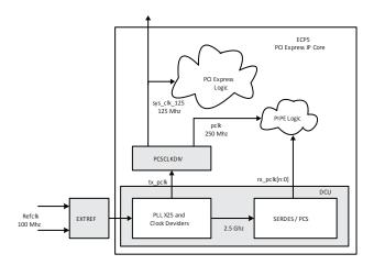
Figure 5.5. ECP5 PCI Express Clocking Scheme
