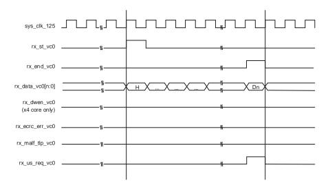
Figure 2.20. Receive Interface, Unsupported Request TLP
