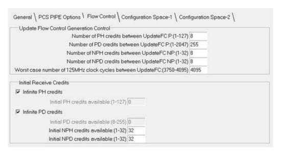
Figure 3.3. PCI Express IP Core Flow Control Options
