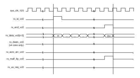
Figure 2.19. Receive Interface, Malformed TLP
