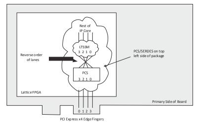
Figure 5.11. Implementation of x4 IP Core to Edge Fingers
