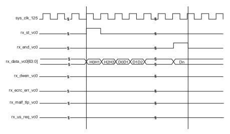
Figure 2.17. Receive Interface, Clean TLP
