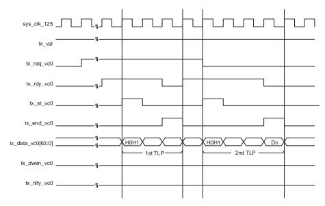
Figure 2.8. Transmit Interface 2.5G IP core Native x4 or 5G IP core Native x2, Burst of Two TLPs
