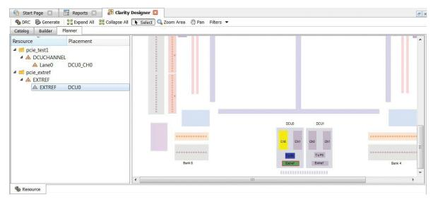
Figure 4.10. Clarity Designer Placed Modules (pci express endpoint and extref)
