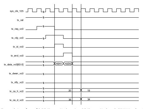
Figure 2.4. Transmit Interface of 2.5G IP core Native x4 or 5G IP core Native x2, 3DW Header, 1 DW Data
