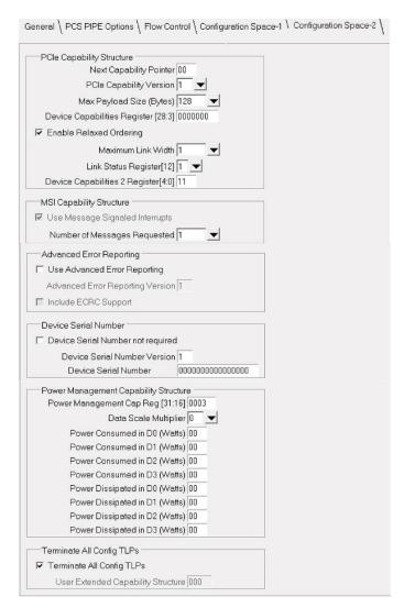
Figure 3.5. PCI Express IP Core Configuration Space - 2 Options
