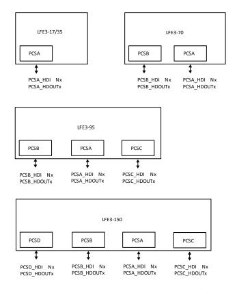
Figure 5.6. LatticeECP3 Device Arrays with PCS/SERDES
