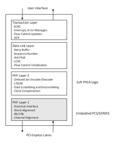
Figure 2.1. PCI Express IP Core Technology and Functions
