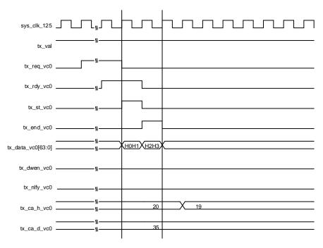
Figure 2.6. Transmit Interface 2.5G IP core Native x4 or 5G IP core Native x2, 4DW Header, 0 DW
