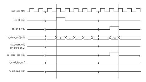
Figure 2.18. Receive Interface, ECRC Errored TLP
