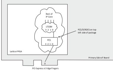
Figure 5.12. Implementation of x1 IP Core to Edge Fingers
