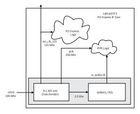
Figure 5.4. LatticeECP3 PCI Express Clocking Scheme
