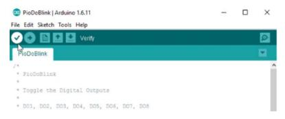
f. The window indicates it is compiling with a progress bar, and when finished, displays **'Done Compiling.'**
