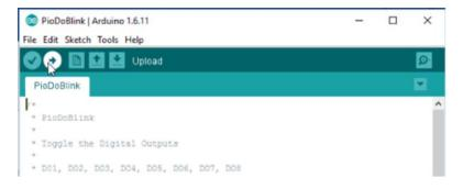
h. After a few seconds the message **'Done Uploading'** is displayed and you can see the LEDs on the board flashing driven by the digital outputs.
