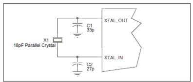
FIGURE 2. CRYSTAL INPUT INTERFACE
