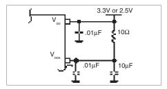
FIGURE 1. POWER SUPPLY FILTERING
