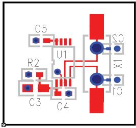
FIGURE 5B. 844031-01 PC BOARD LAYOUT EXAMPLE
