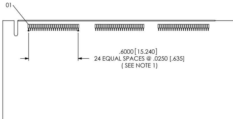
BROKEN EDGE MUST BE LOWER THAN PLATED EDGE OR MILLED FOR HOUSING CLEARANCE.
