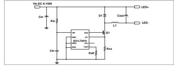
**Note:** In the above configuration, it is important to pay attention to the VGSON value for Q1. IS31LT3918 provides a maximum gate drive of 4.5V (typ), thus requiring that a low threshold voltage NMOS be used.
