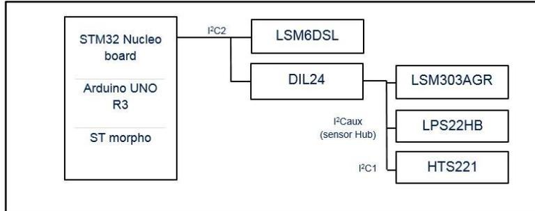
**Mode 5: LSM6DSL plus I<sup>2</sup>C sensor hub DIL24**
