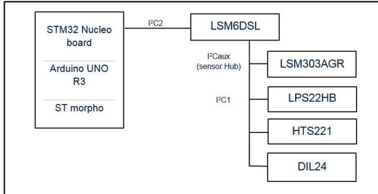
**Mode 3: DIL24 plus LSM6DSL I<sup>2</sup>C sensor hub (all sensors)**
