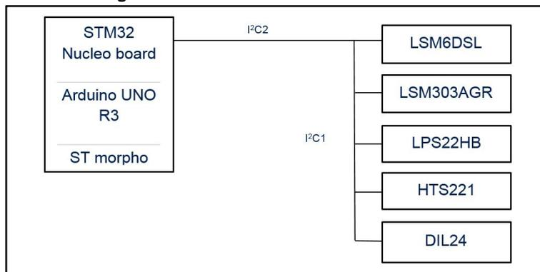
**Mode 2: LSM6DSL I<sup>2</sup>C sensor hub (all sensors)**
