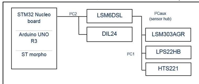
**Mode 4: LSM6DSL plus DIL24 I<sup>2</sup>C sensor hub (all sensors)**
