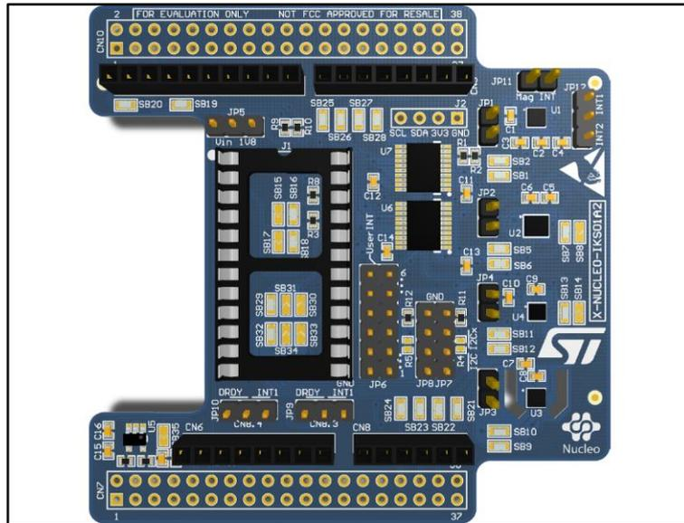
Figure 14: X-NUCLEO-IKS01A2 bottom side layout
