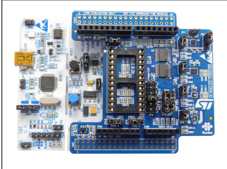
The X-NUCLEO-IKS01A2 must be plugged on the matching pins of the STM32 Nucleo board connector.
