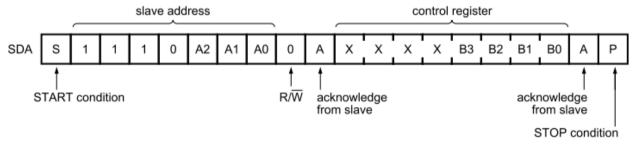
Figure 11. Write Control Register
