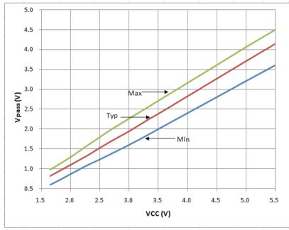
Figure 6:Vpass voltage VS Vcc
