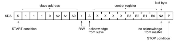
Figure 12. Read Control Register
