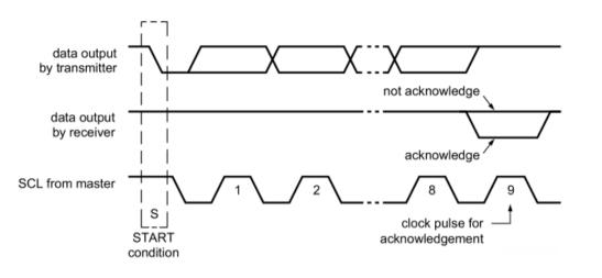
Figure 10. Acknowledgment on I2C Bus
