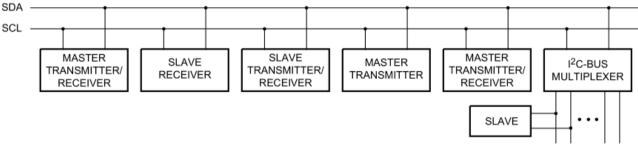
Figure 9. System Configuration
