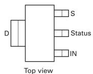
**Note:** The tab is connected to the drain pin and must be electrically isolated from the source pin. Connection of significant copper to the tab is recommended for best thermal performance.
