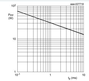
Fig. 7. Peak pulse power as a function of exponential pulse duration; typical values
