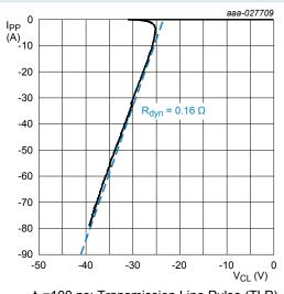
t<sub>p</sub>=100 ns; Transmission Line Pulse (TLP)
