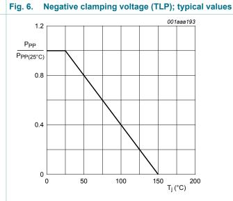
Fig. 8. Relative variation of peak pulse power as a function of junction temperature; typical values
