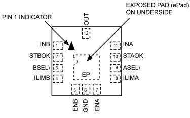
12-Pin 2mm × 2mm FTQFN (FT) (Top View)
