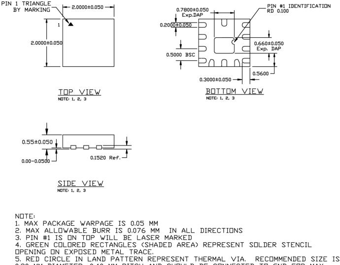
0.20 MM DIAMETER, 0.40 MM PITCH AND SHOULD BE CONNECTED TO GND FOR MAX THERMAL PERFORMANCE 6. PURPLE HIDDEN LINES ARE RECOMMENDED METAL TRACE/GND PLANES FOR IMPROVED THERMAL PERFORMANCE
